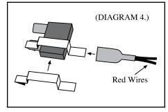
wires for ground. A good ground connection is important. Locate a screw that is in an unpainted metal material for grounding.
