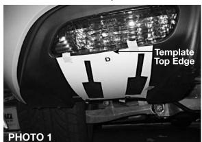
**STEP 1.** Using supplied mounting templates attach Driver side template (marked D) onto rear lower body panel. The (2) holes in template will locate on the (2) plastic round push-in style fasteners located in lower body panel. Line up top edge of template with lens opening. Use masking tape to hold template in place. SEE PHOTO 1
