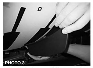
**STEP 3.** Remove red liner from tape on (1) Diffuser. Start by locating Diffuser for positioning as far forward (toward front of car) as possible. The overall fit is best when Diffusers are mounted as forward as possible into die cut template. SEE PHOTO 3 As you position Diffusers make sure they locate correctly into template centered in narrow fin area.
