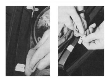
2. **IMPORTANT.** Thoroughly clean the mounting surfaces on the body nacelle and mounting brackets. use glass cleaner such that no dirt or oily film exists on either surface. **DO NOT** touch surfaces after cleaning.
