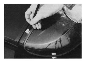
1. Place masking tape on the headlight nacelle opposite the holes on each lense prior to marking centers. Then fit the rubber trim around the lenses, tape them in place and mark each hole's location on the nacelles. Be sure to mark **DIRECTLY ACROSS** from each hole as shown. Z cars utilize 3 holes per lens and ZX cars 4.
