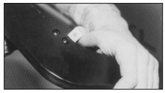
Install mounting tabs on each guard using (2) 3/8" phillips machine screws and (2) kep nuts. Bend tab so it will lie flat on lower fender surface.
