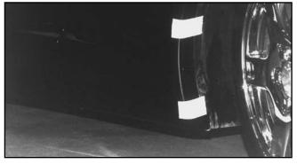
Hold guard up to fender in position. Note: masking tape should be applied for marking holes to drill. Apply tape to fender well. Holding guard in a perfect level position, mark through holes in guard onto tape. A helper can assist in aligning per diagram A.
